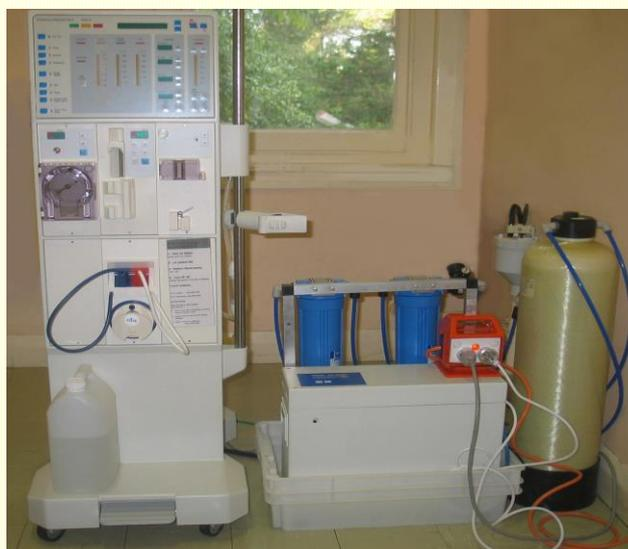
Figure 1, Haemodialysis machine & reverse osmosis machine
